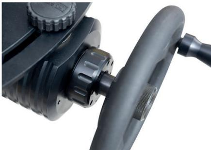
With the MOCA25 wheels you can control the pan and tilt movement of the Remote Head. The wheels are optimized for this particular application in terms of weight and synchronization. The friction can be individually adjusted for both wheels of the pan and tilt axis to produce the desired resistance.
